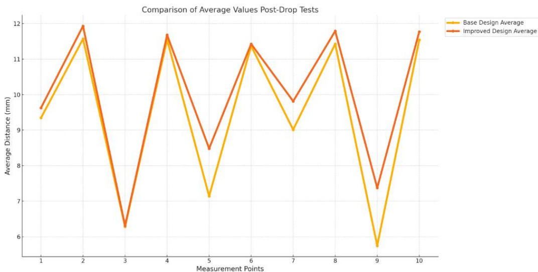
Figure 19. Baseline design and post-Improved design drop test door distance measurement average results comparison in chart
