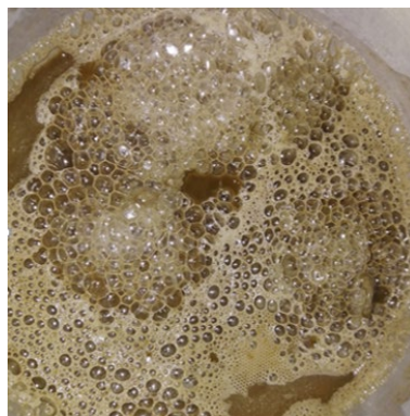
Figure 3. Formation of stable air bubble from pure lignin
