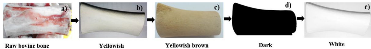
Figure 2. Illustration the color of bovine bone changes during the calcination process
