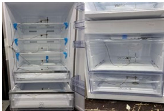
Figure 1. Photos of thermocouple positions on a sample
