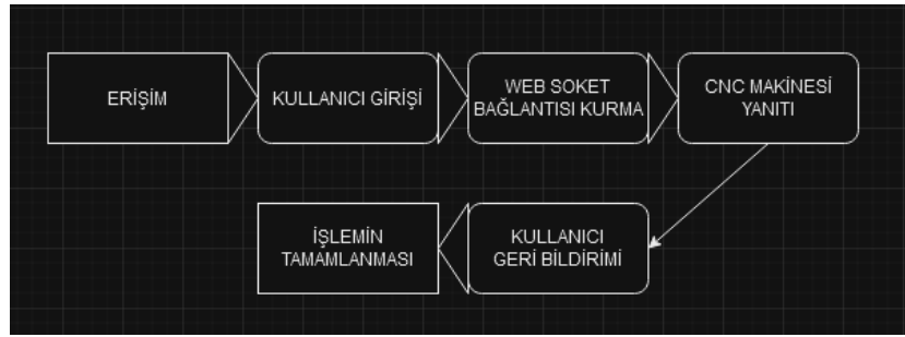
Figure 7. Websocket flow diagram
