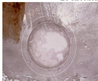
Experimental Number 1: 1.22±0.3 (1500 rpm, 200 mm/min)
