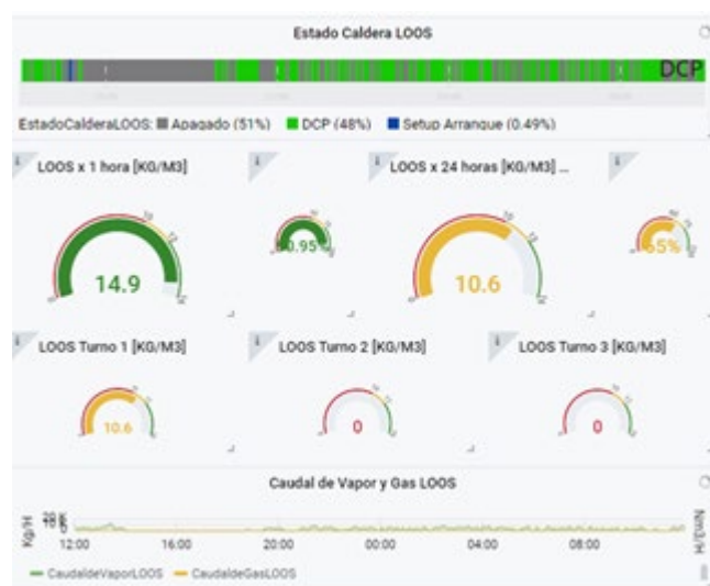
Figure 3. Dashboard that shows the status of a boiler from data gathered by the IIoT architecture
