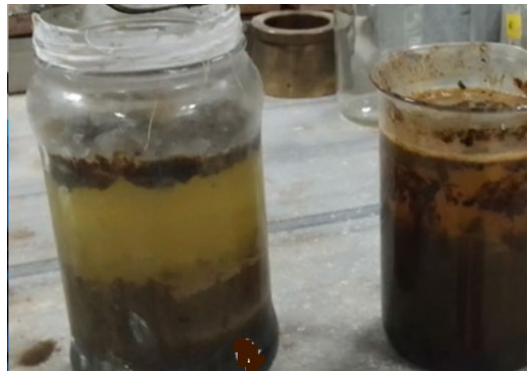
Figure 2. Obtaining pure lignin from liquor by precipitation process
