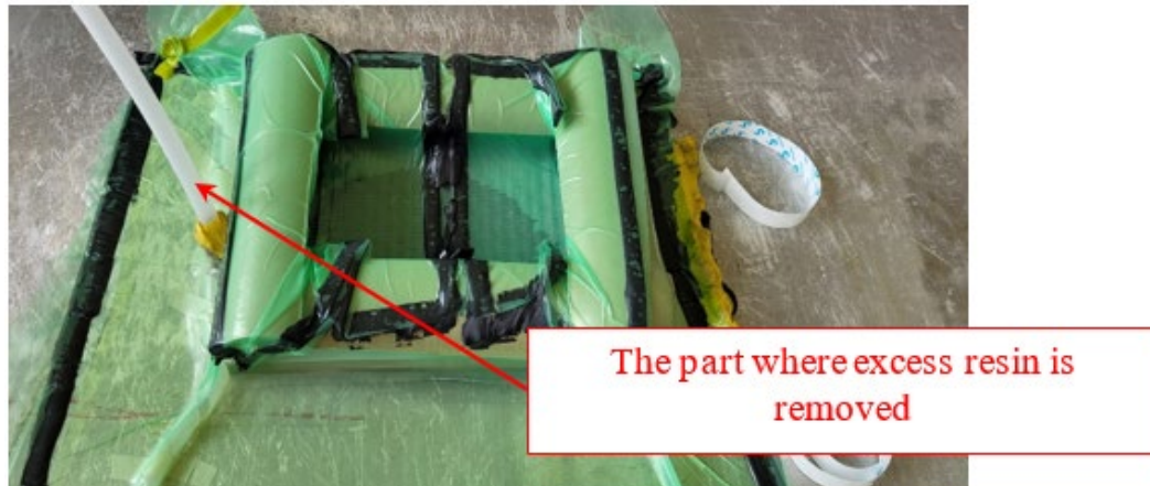
Figure 6. Removing excess resin from the mold
