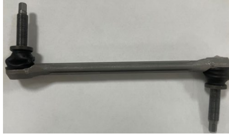
Figure 9. Stabilizer link part produced with SLM
