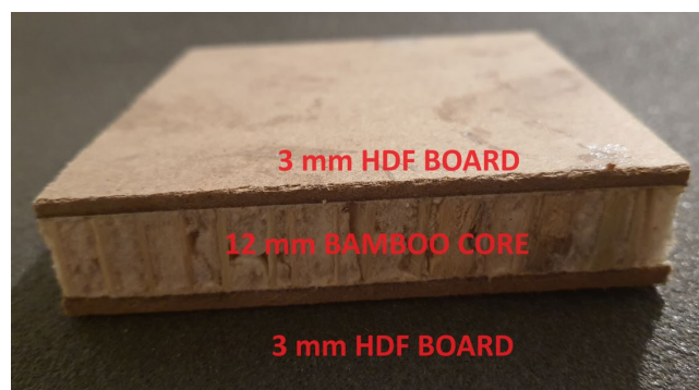
Figure 1. Bamboo based composite side sectional view
