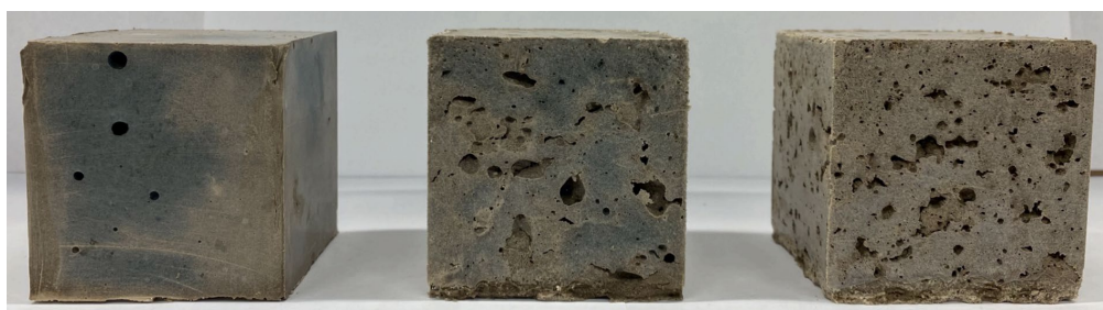
Figure 6. Cubic geopolymer samples containing recycled polyurethane powder (rPU). From left to right, rPU loading factor is 0%, 5% and 10% by weight [21]
