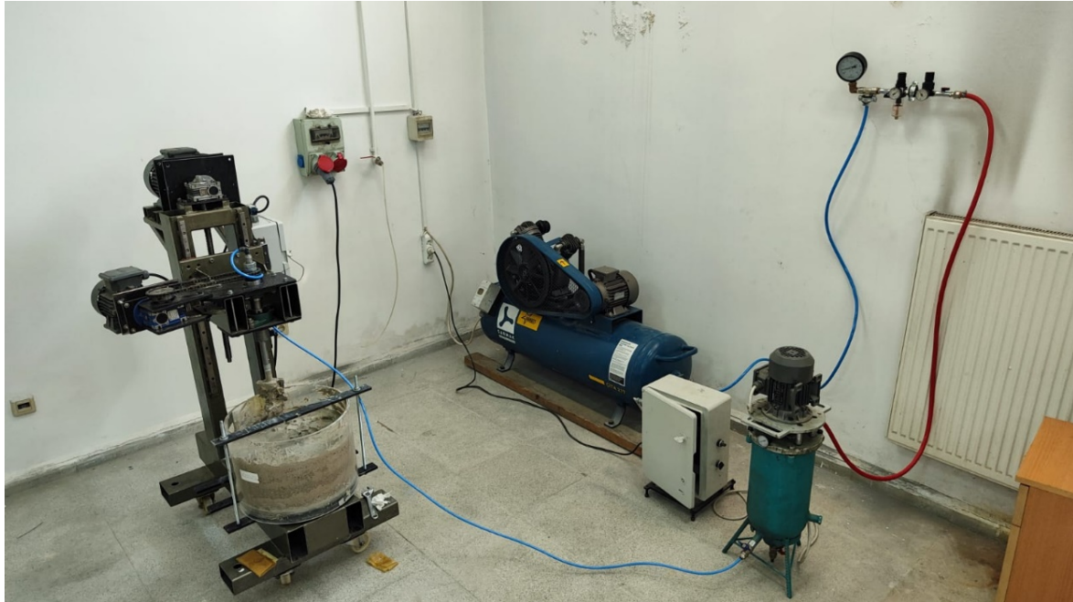
Figure 1. Small scale deep mixing system
