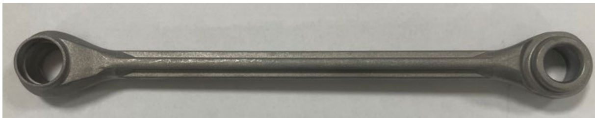
Figure 5. EN AC 43200 stabilizer link body manufactured with aluminum injection
